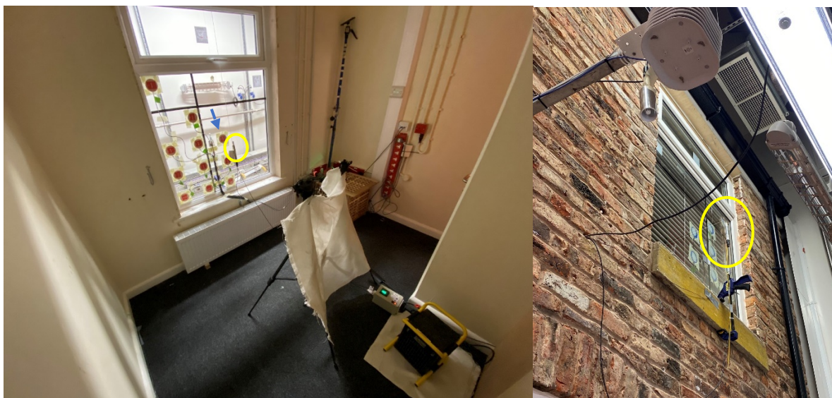
Figure 1 - a) Internal test setup, with internal temperature sensor circled in yellow and centre pane HFP denoted by the blue arrow. b) Shows the external temperature sensor highlighted in yellow.
