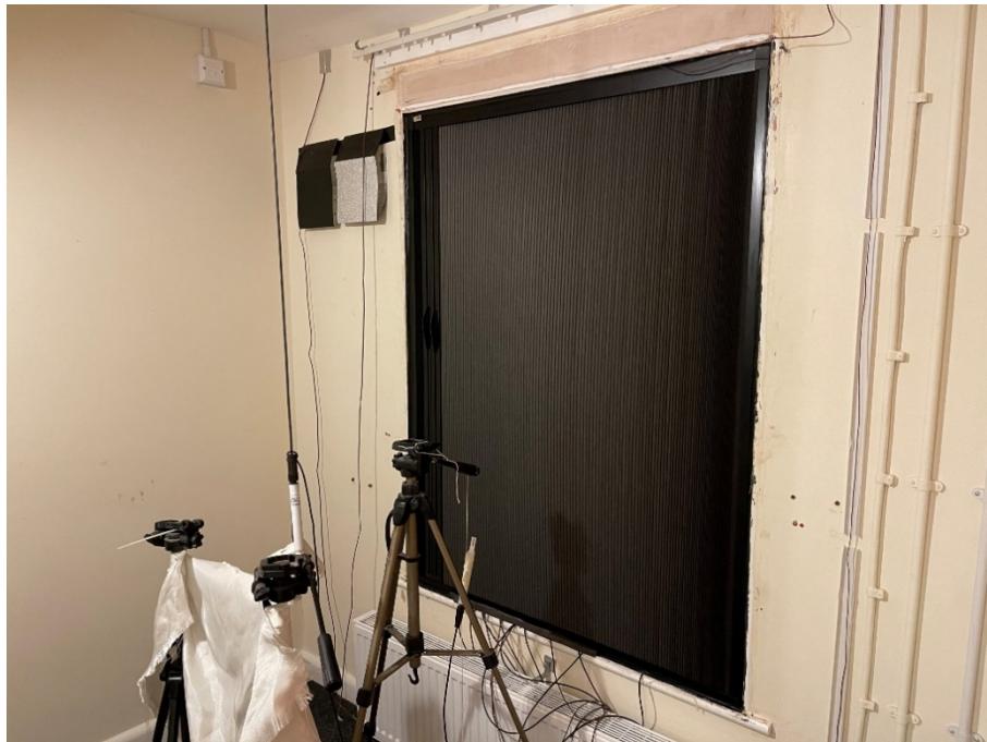
Figure 4 – Experiment set-up for the Sheer Intimacy and Light Seal.
