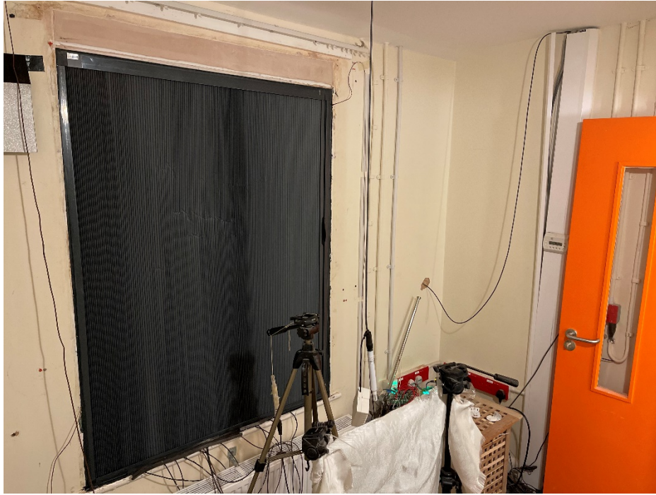
Figure 7 – Test set-up for 02 Single Light Seal.
