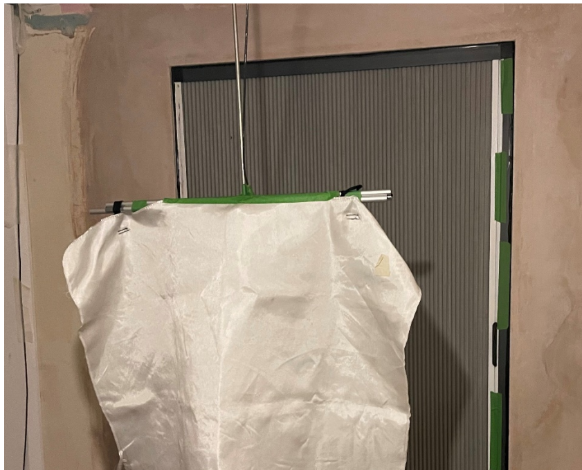
Figure 6 – Single glazing test set-up for Double Duette.
